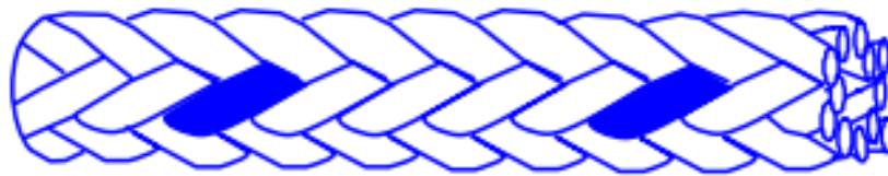
Figure 5.7: Braided tether (Bosman et al., 2013)
