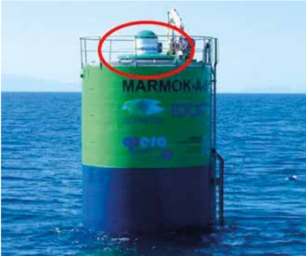
Biradial turbine installed on MARMOK-A-5 spar-buoy OWC, at Bimep, Basque Country, October 2018 (left). Model of UGEN at the wave tank of Plymouth University, UK (right).
