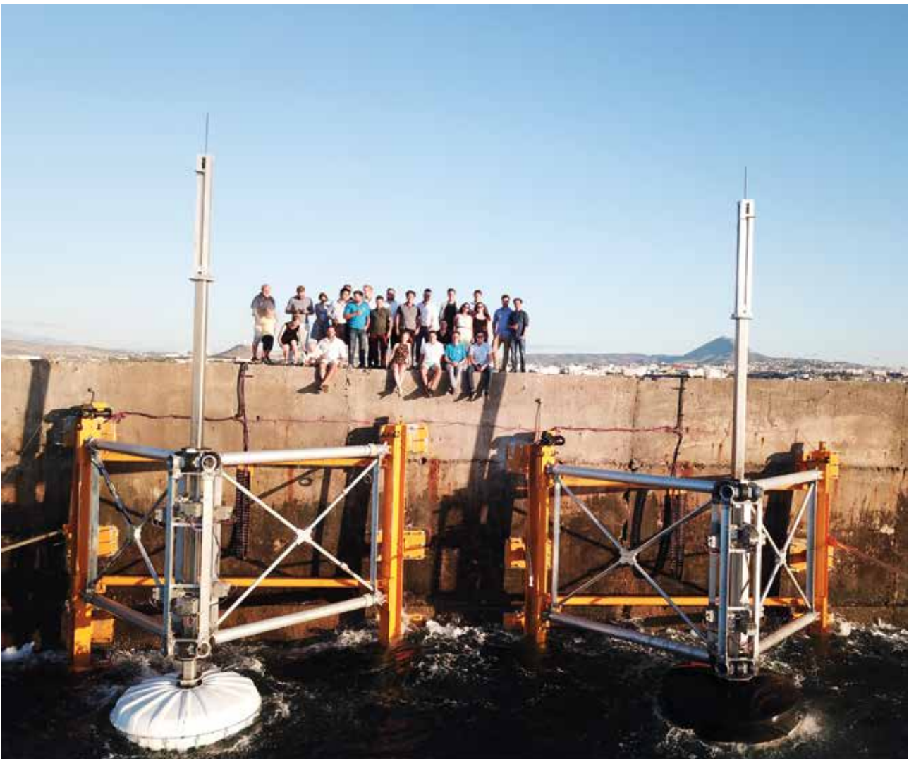
Second generation SINN Power WECs at the port of Heraklion, Greece
