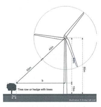
where: bl = blade length, hh = hub height, fh = feature height (all in metres). For the example above, b = 69.3 m.
