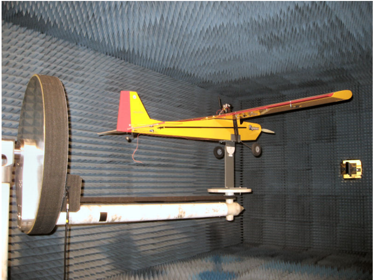
Figure 38. Model aircraft used as test target mounted on the swivelling table on the measurement tower in the anechoic chamber. The radar antennas are in the window to the right in the picture. Photo: Yngve Steinheim.
