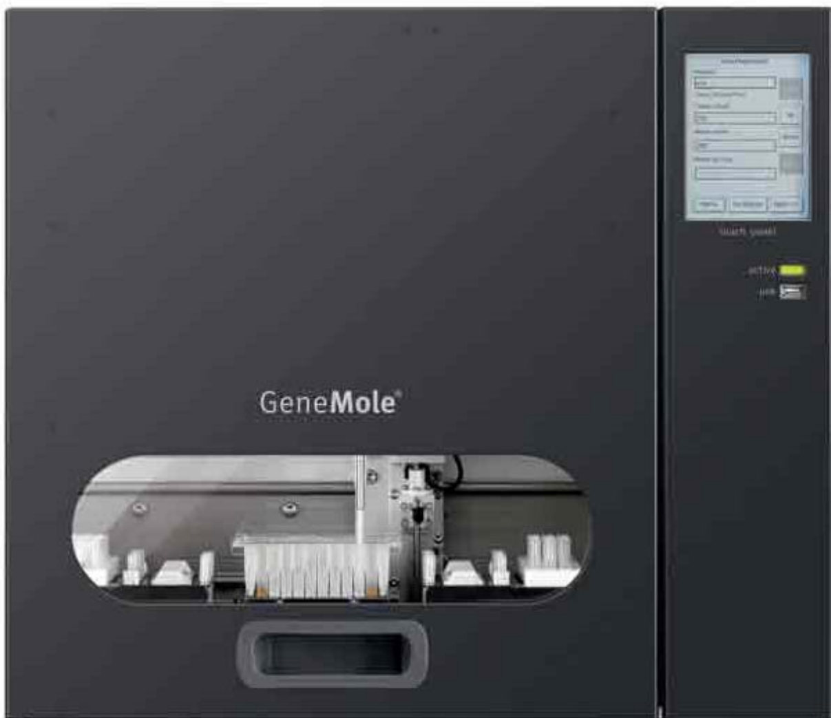
Figure 21 The GeneMole instrument, which has now been implemented in the project to streamline the production of DNA-data from feathers and tissue of dead eagles.
