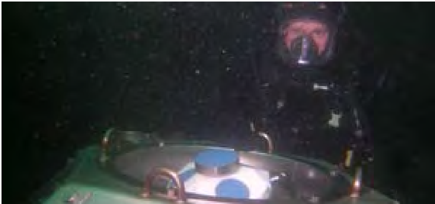
Spot ADCP deployment
