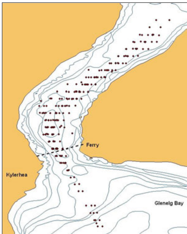
Figure 6. Kyle Rhea and northern Sound of Sleaf and 228 acoustic sampling stations (separated in latitude by 150 m). The ferry track is also shown (dotted line) where the strait is narrowest (300 m).
