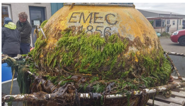
Figure 3. Datawell DWR MkIII data buoy with approximately 12 months accumulation of biofouling from the EMEC wave test site at Billia Croo, Orkney.
