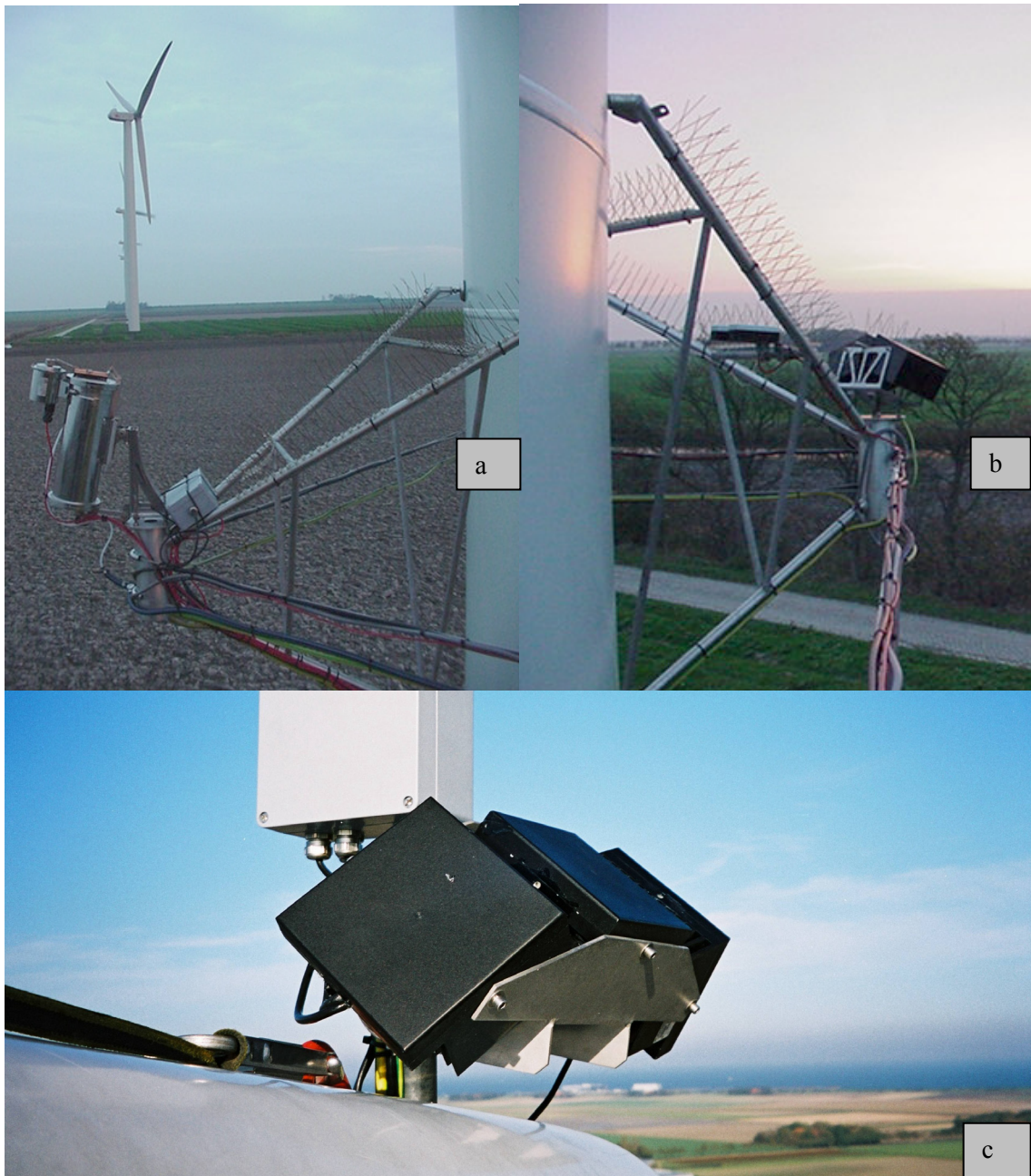
Figure 5: Outdoor equipment of the WT-Bird prototype on Nordex N80 turbine at EWTW
