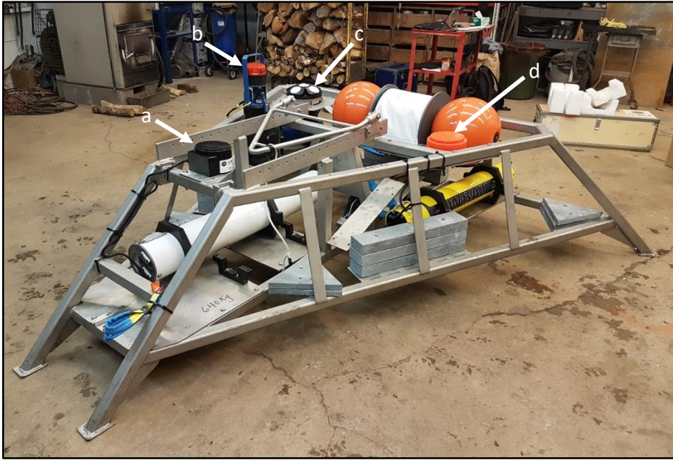
Figure 2. FAST3 platform prior to deployment at the FORCE test site. (a) ASL AZFP transducer; (b) Aanderaa SeaGuard RCM; (c) Nortek Signature 500; (d) Simrad EK80 WBAT transducer.
