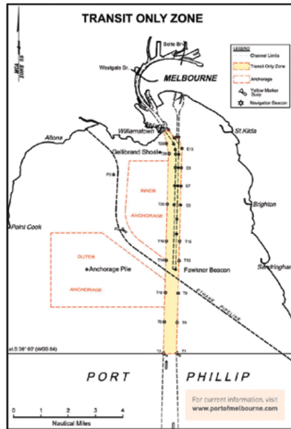
Figure 12.6 Transit only zone in Port Phillip Bay. Also shown are the two anchorages used by ships waiting for berths in the port to become available
