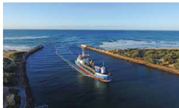
The Tommy Norton trailer suction hopper dredge is used to maintain ocean access to Bass Strait. Photo: Gippsland Ports
