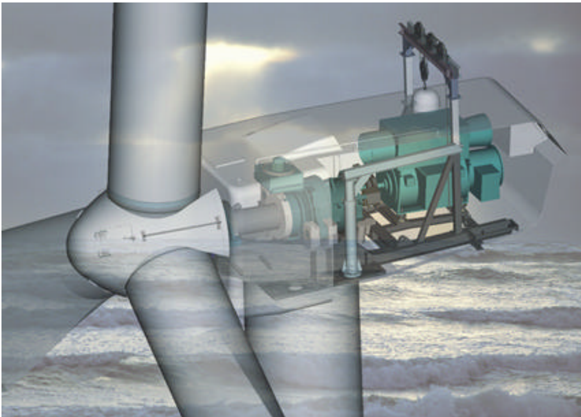
Figure 6 Turbine interior, service crane mounted
