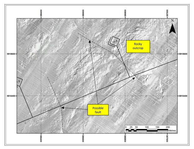
Figure 11: Large rock outcrop beneath route centre line between KP10.173 and KP11.016
