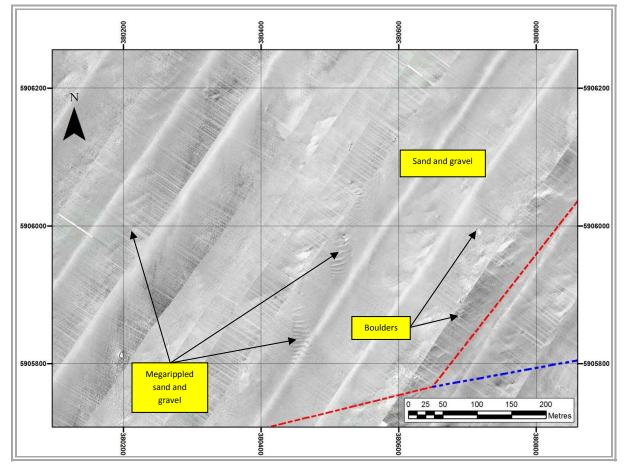
Figure 3: Seabed sediment distribution within the PDA
