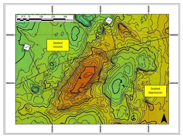
Figure 8: Seabed depression and ridge to south of route between KP13.0 and KP14.0
