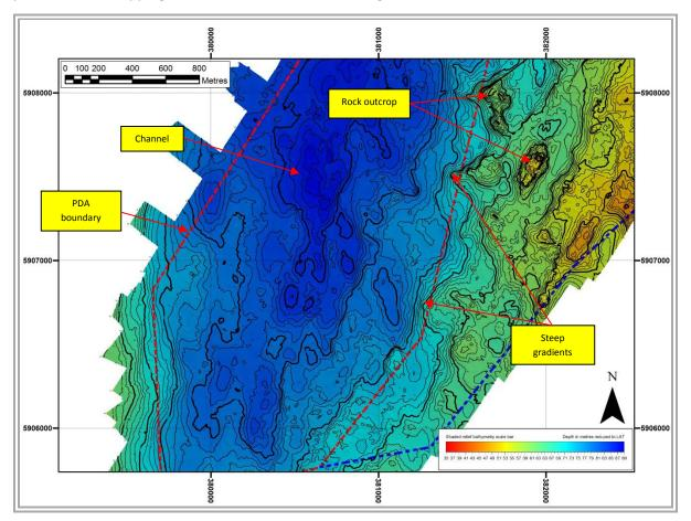
Figure 2: Shaded-relief image showing seabed channel orientated north-northeast to south-southwest
