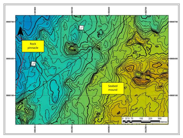
Figure 9: Seabed mounds and rock pinnacles at north-eastern edge of channel feature
