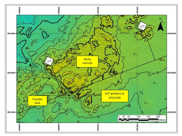
Figure 7: Shaded-relief image of rocky area between KP10.175 and KP10.600
