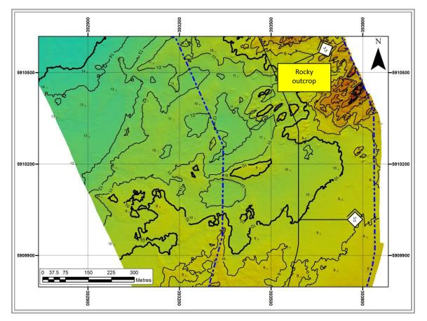
Figure 6: Shaded-relief image between KP3.000 and KP3.5000
