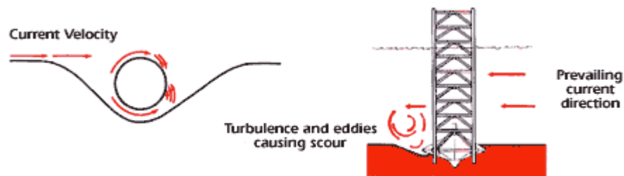
Figure 6 - The formation of scour, taken from Website 5
