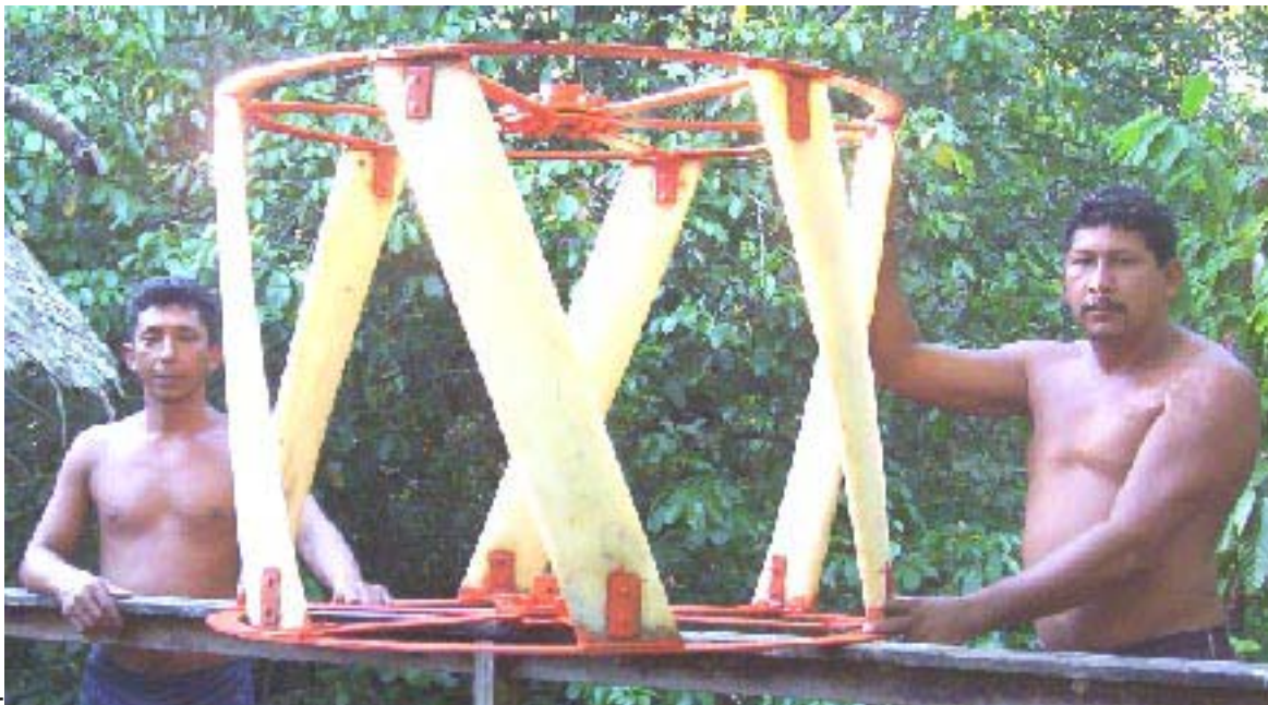
Rural artisans assembled, installed, and operate this 6-blade Gorlov Helical Turbine
