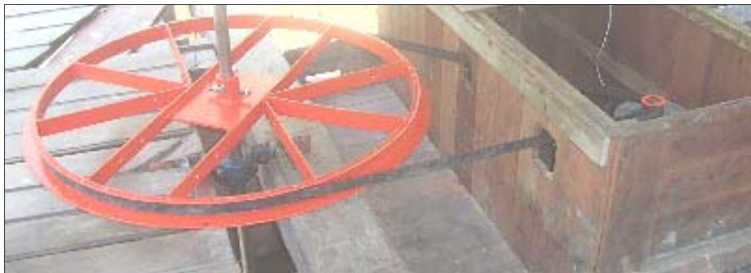
Pulley, 1.08 m (43 in) in diameter, and belt
