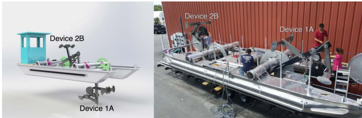
Figure 3. Schematic and photo of the second Leading Edge prototype with two devices, each with two rows of hydrofoils. Photo credit Michael Miller.
