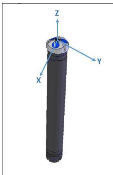
Figure 1. Beam geometry of Aquadopp Profiler used during the tests (courtesy of nortek.com).
