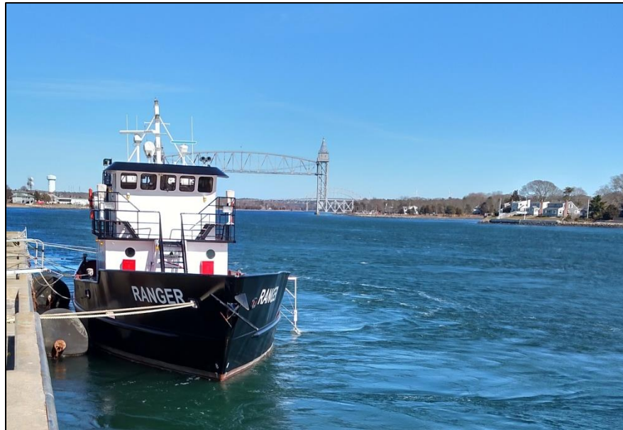
Figure A-1: Photograph looking eastward of the MMA M/V Ranger with pole mount off outboard rail. The Aquadopp profiler transducers were positioned approximately 16" below the surface. Stabilizer lines ran fore and aft to minimize vibrations. This photo was taken Saturday afternoon during strong westerly winds.
