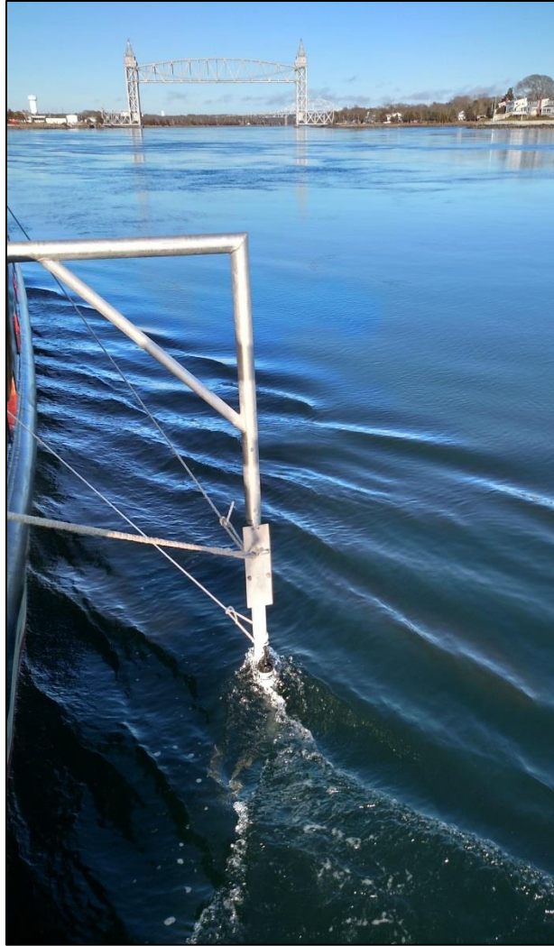
Figure A-2: Close-up of the Aquadopp profiler mounting. This photo was taken during an ebb (westerly) tide March 11, 2016 approximately 16:04 hours, just after installation. Note the strong wake coming off the instrument and mounting pole. Surface currents were measured to be 1.33 meters/second at this time (2.6 knots). Also note the relatively smooth water surface reflecting calm wind conditions, in contrast to the brisk winds of Figure A-1.
