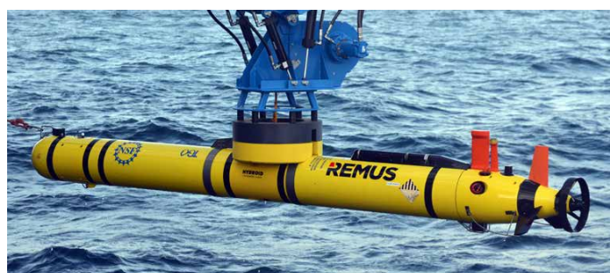
FIGURE 13. (left) Coastal gliders are staged on deck for pre-flight checks via satellite telemetry to the shore lab. (right) An AUV is prepared for deployment using a hydraulic launch and recovery system fitted to R/V Neil Armstrong. Credit: OOI Pioneer Array Program, Woods Hole Oceanographic Institution
