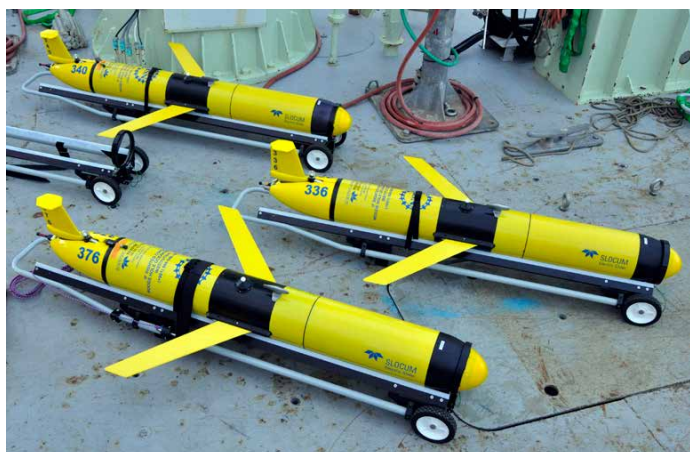
FIGURE 13. (left) Coastal gliders are staged on deck for pre-flight checks via satellite telemetry to the shore lab. (right) An AUV is prepared for deployment using a hydraulic launch and recovery system fitted to R/V Neil Armstrong. Credit: OOI Pioneer Array Program, Woods Hole Oceanographic Institution
