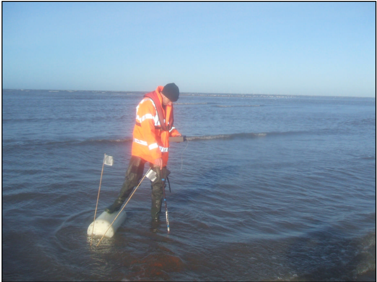
Figure 20. EMF Measurements at Rhyl (North Hoyle Wind Farm). The Hand-held iE field sensor is submerged in front of the surveyor's left foot and provided real-time data via a visual display. The pod (silver/white barrel) contained both B and iE field sensors and had logging capability but provided no live data. The two flags marked the position of the cable as detected by the hand held sensor and a magnetometer.
