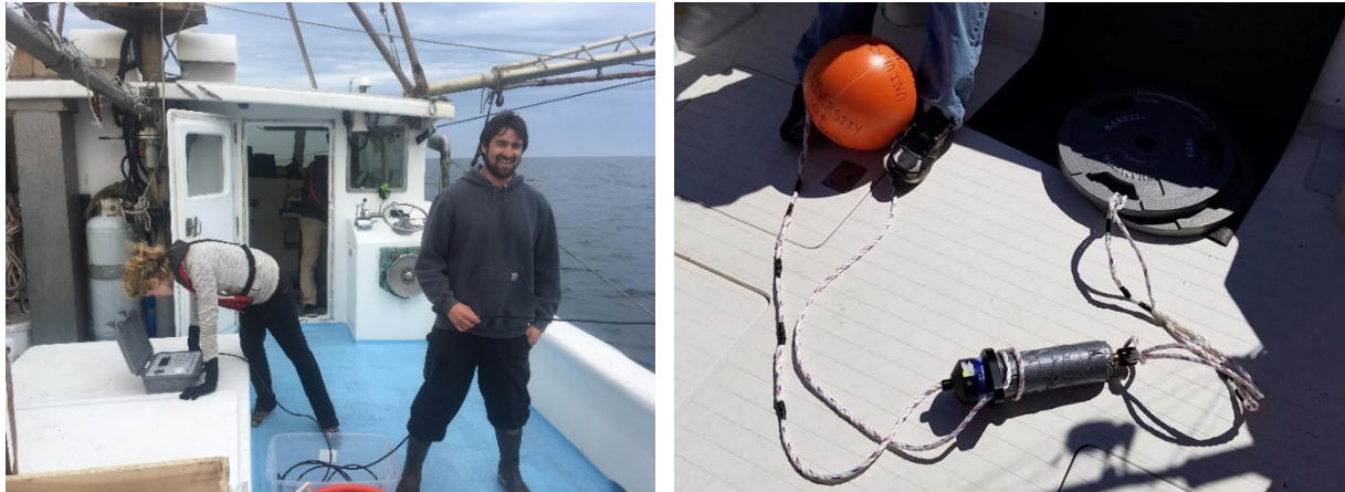
Figure 4. Acoustic Release receiver detection (left) and acoustic release mooring design (right).
