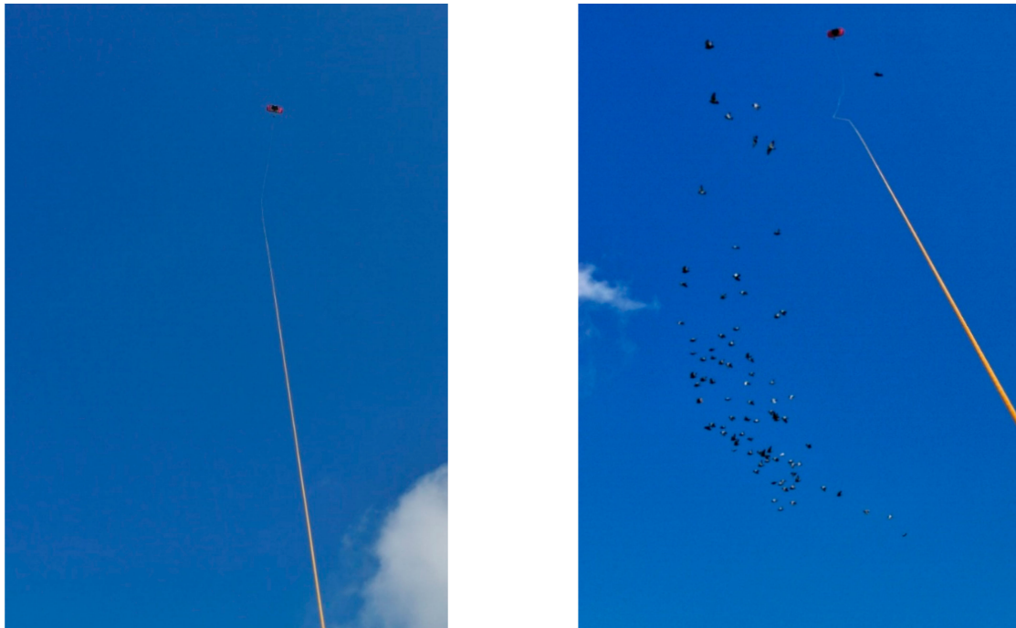
Figure 5. Pilot operation of the 20 kW kite power system of TU Delft [88] before ( left ) and after a bird collided with the tether ( right ). The bird continued the flight seemingly unaffected, which suggests that bird collisions with a tether are possible but do not necessarily have to be fatal. Max Dereta took the photos on 28 June 2011 at Valkenburg airfield, The Netherlands.
