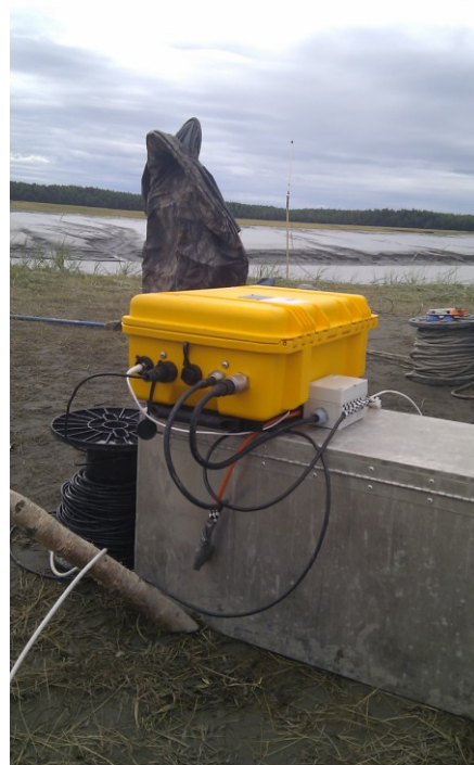
Figure 2. The Pelicase based PAMBuoy® system used for the 2012 trials.
