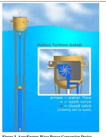
Figure 3. AquaEnergy Wave Power Conversion Device
