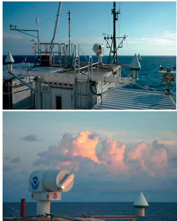
FIG. 1. (top) Instrumentation deployed on the *RHB*, including the lidar seatainer. (bottom) Doppler lidar scanner (left part of photograph), probing the atmosphere in the conical scan mode, and GPS housing (bottom-right part of photograph).
