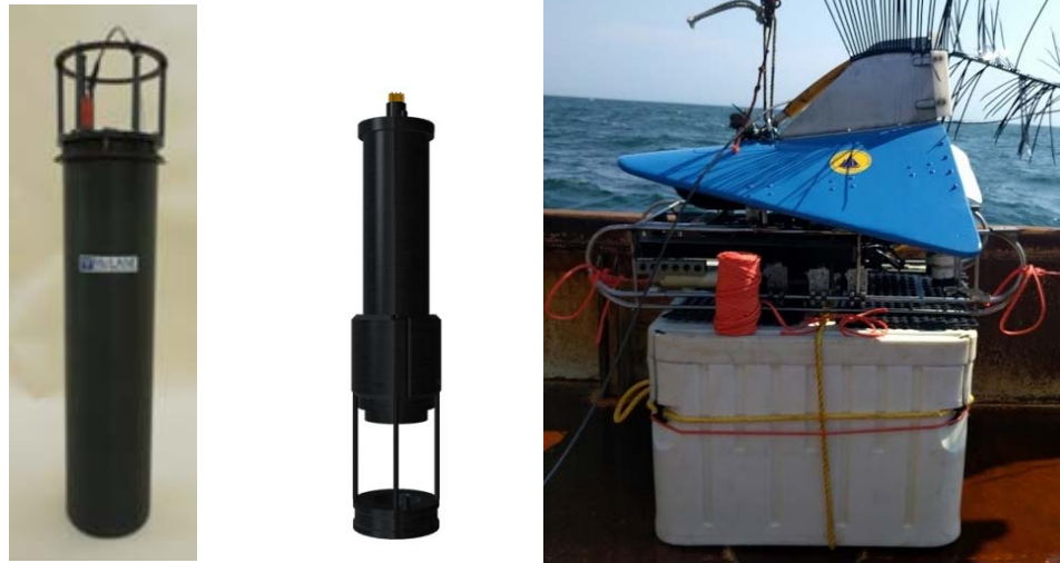
Figure 1. Examples of new technologies for automated in situ microscopic imaging of marine plankton and benthic habitats. Left: Imaging FlowCytobot, optimized for imaging single-celled primary producers (phytoplankton) and protozoa; Middle: CPICS, optimized for imaging secondary producers (zooplankton) and marine aggregates; Right: HabCam benthic stereo-imaging vehicle, optimized for imaging surveys of benthic environments.
