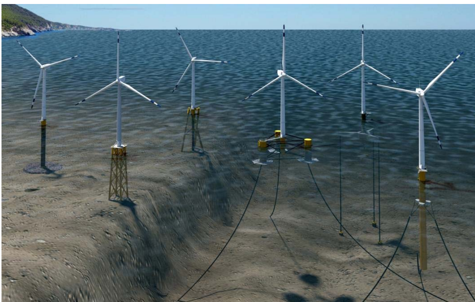
Figure 2: Cartoon of the various types of potential foundations available for offshore wind energy installations. Image credit: NREL.
