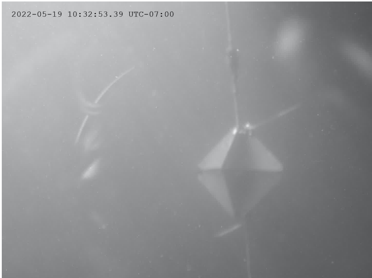
Figure 11. BF display showing RR target just before it is pulled from the water at the end of the test run.
