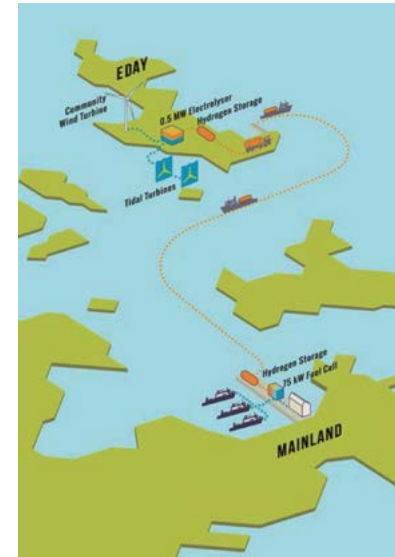
Fig. 1. First hydrogen gas produced from tidal power at test site of EMEC in the Orkney Islands [5]
