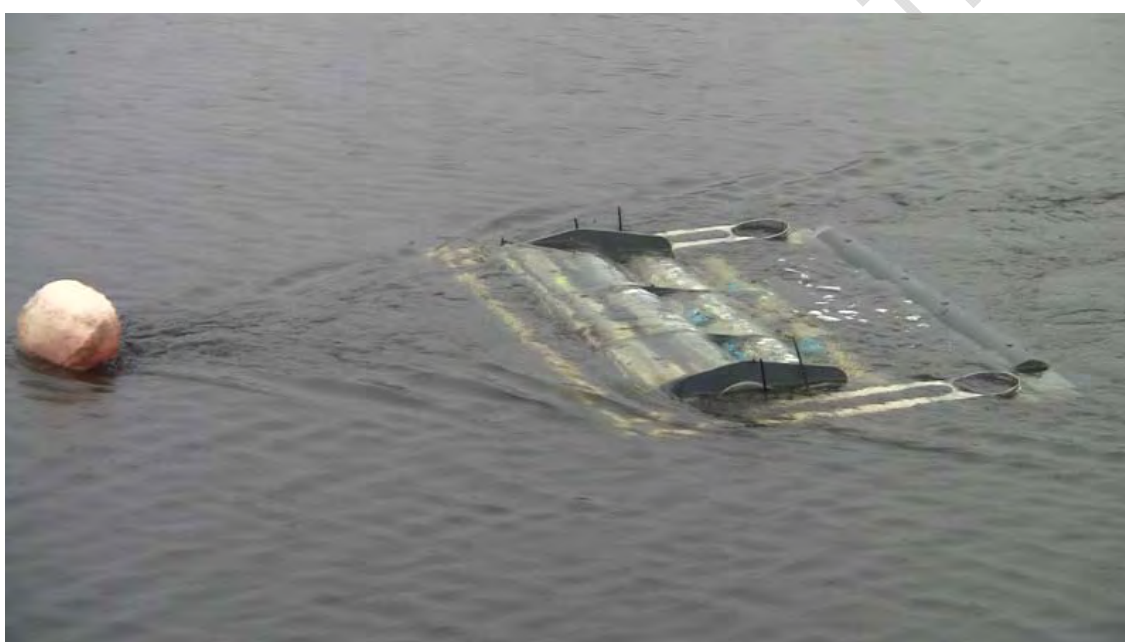
Figure 6: Scale Model Oyster 2a WEC in Closed Position being wet towed
