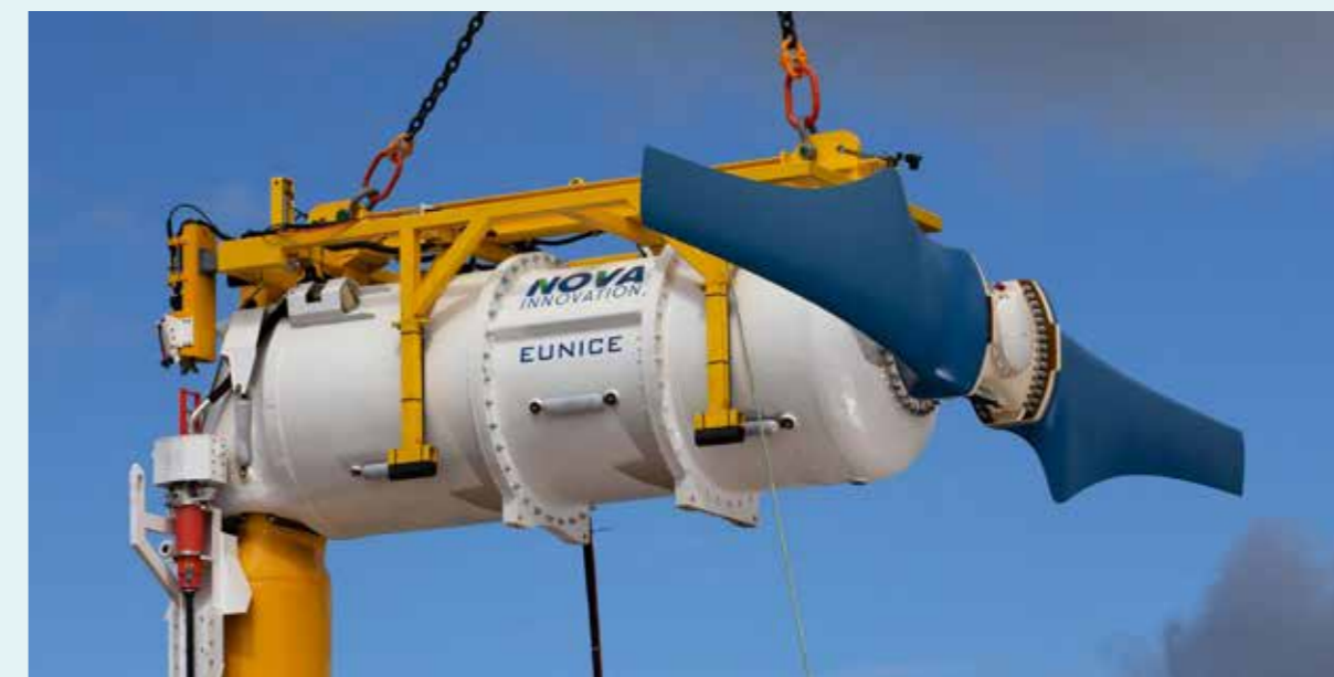
The 'EUNICE' tidal turbine (Source: Nova Innovation)
