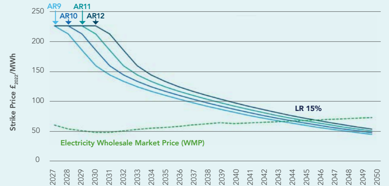
Figure 21 – Strike price trend associated with achieving 6GW of wave by 2050 when there are delays to cost reduction at a 15% learning rate
