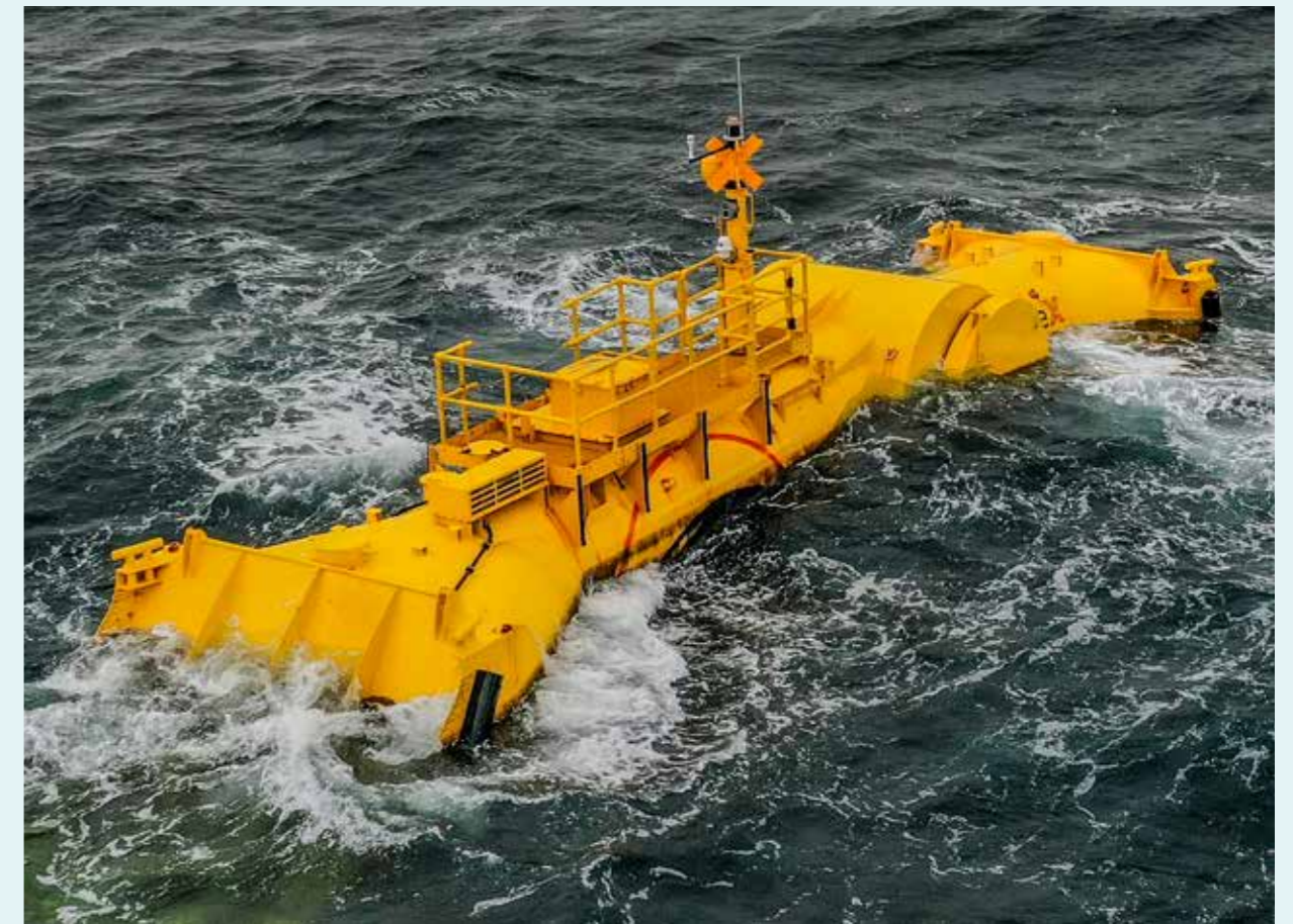
Mocean Energy Blue X wave energy converter in operation at EMEC Scaapa Flow test site (Source: Mocean Energy)
