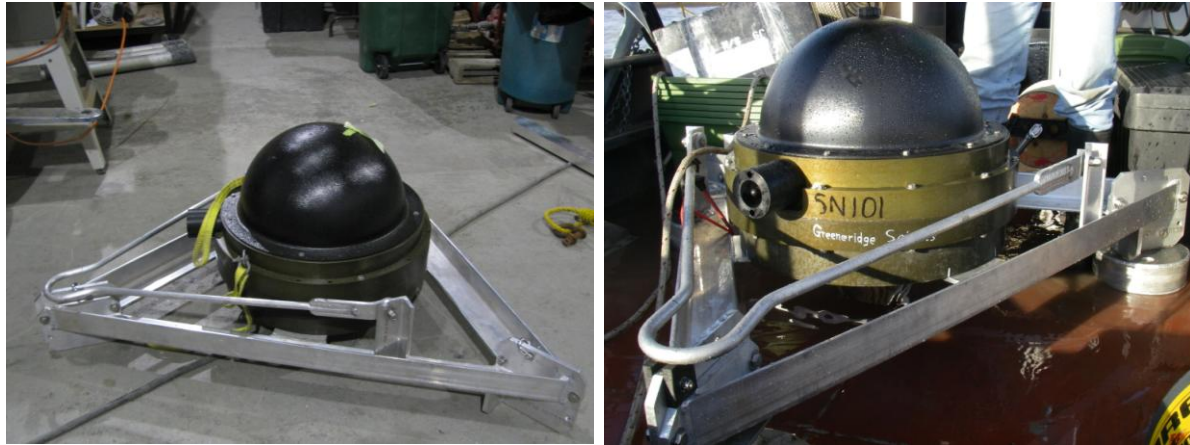
Figure 2. Cook Inlet DASAR and mooring frame, left. Ready for deployment onboard vessel, right.
