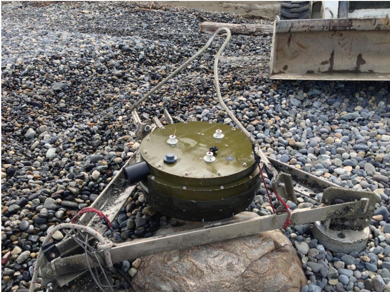
Figure 18. DASAR SN 101 after recovery on June 24, 2013, eight months after deployment at East Foreland showing damages including lost ABS cover, missing two of three hydrophones and bent mooring frame.
