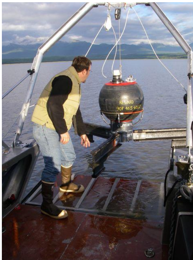
Figure 19. EAR and C-Pod in prototype mooring used by Team CIBA in Cook Inlet with PAM devices housed in buoyant portion of pop-up buoy system.
