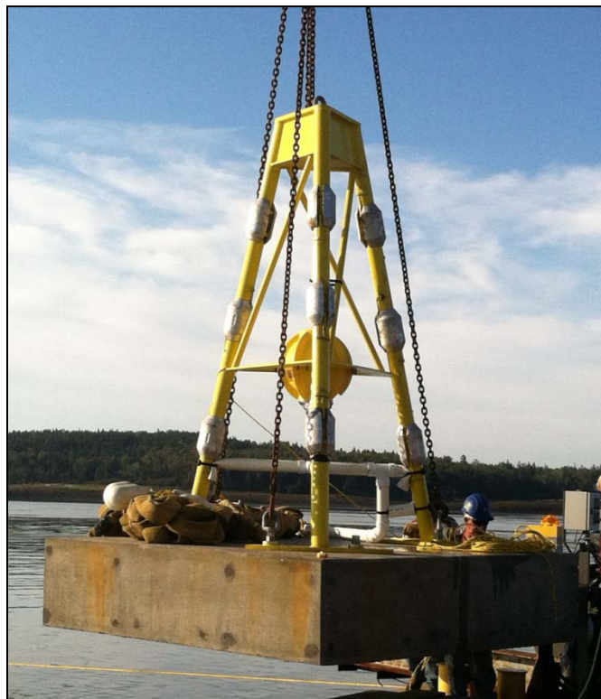
Figure 19. Simrad environmental monitoring observation tower
