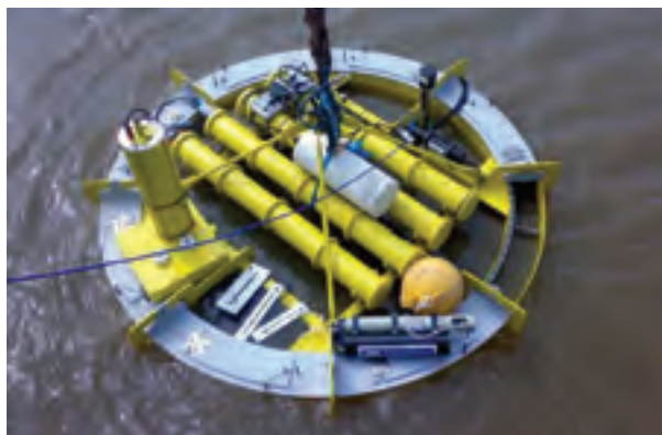
Figure 1b: Photograph of the flume partially submerged during recent field trials. A section of the lid has been removed in order to ascertain paddle movement visually. At 5 o'clock a pop up buoy with acoustic release is shackled to the instrument frame.
