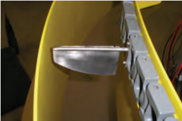
Figure 3: Photograph showing one of the 8 paddles mounted within the annulus and affixed to the chain-drive.
