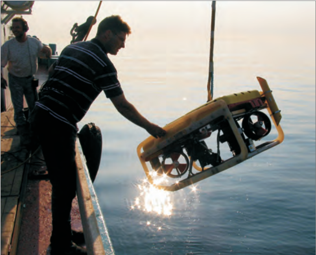
Figure 3: Launching the ROV. Note the USBL transponder attached to the rear of the ROV
