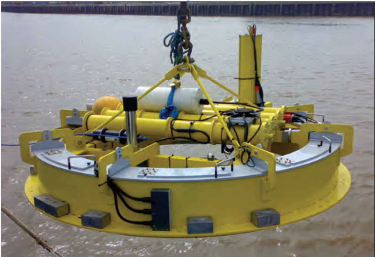
Figure 1a: A wide angle shot of the flume instrument. The long yellow pods on the top of the instrument house the batteries and Arctic motor control software. The white pod directly atop the instrument is the data logger. On the outside channel facing is the housing for 3 optical backscatter turbidity sensors placed at different heights. The vertical steel unit is a height adjustable corer.
