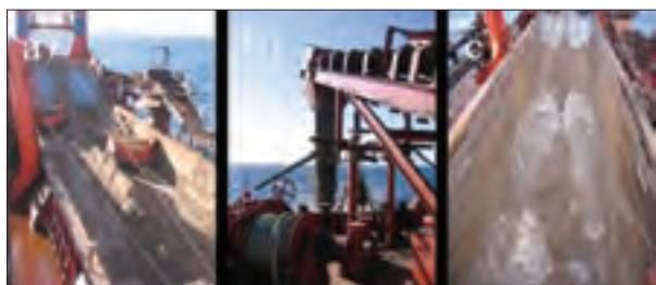
Figure 3: a) buckets moving material into hopper at the stern of the vessel during 'dry' discharge. b) material being deposited over the stern of the vessel during 'dry' discharge. c) flooding of the cargo hold following opening of hold doors during 'wet' discharge of remaining cargo.
