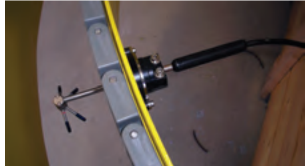
Figure 5: Photograph of the Nortek ADV current velocity/altimeter sensor. The instrument is 'downward-looking' and acquires velocity data approximately 10cm above the bed.
