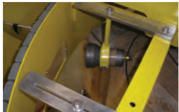
Figure 6: Photograph showing the window in the inner wall and the two LED lamps. The camera [not shown] is out off the shot just to the right.
