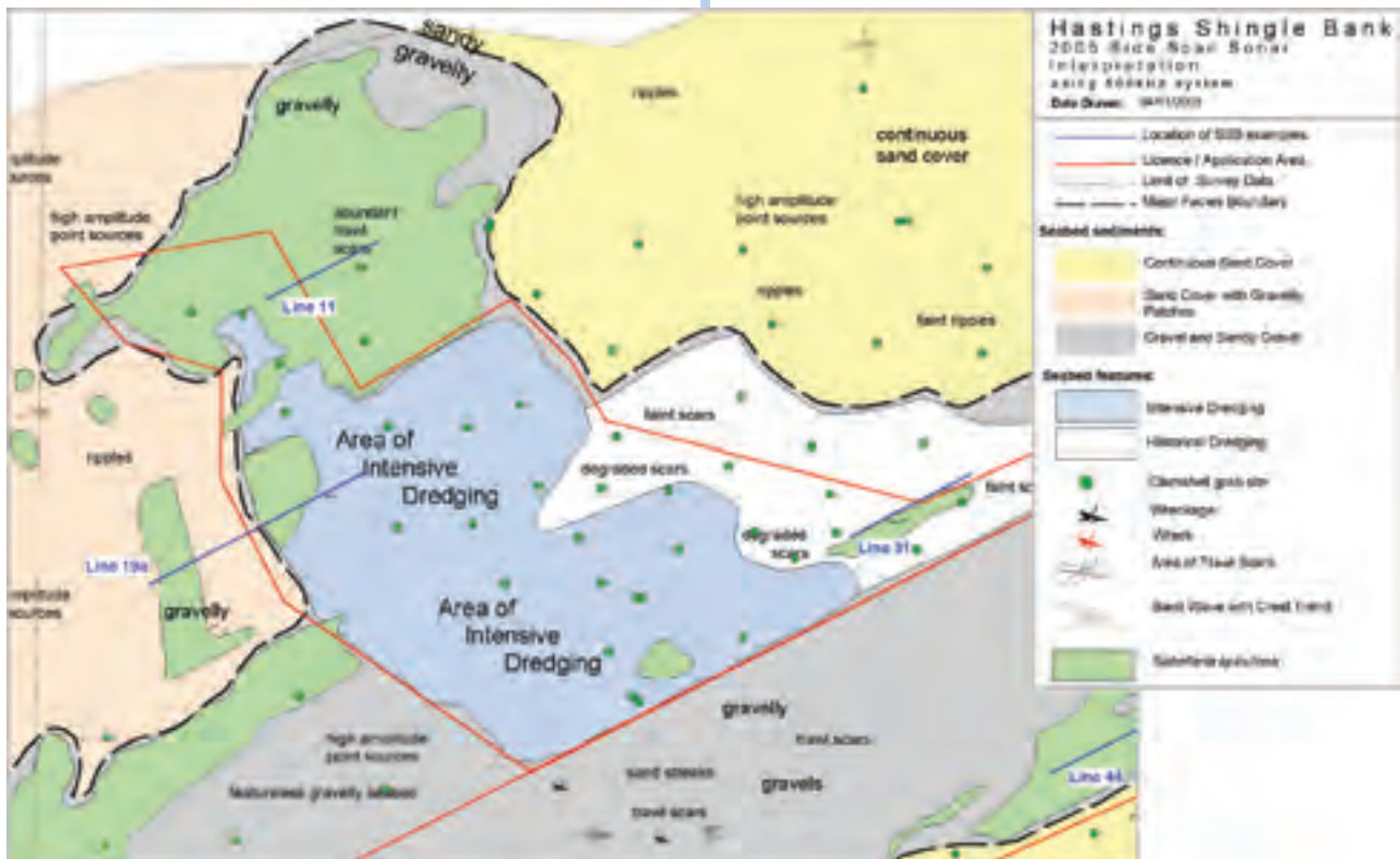
Figure 1: Chart section of the study site showing the June-July 2005 Side Scan Sonar interpretation carried out by the Resource Management Association (RMA) as part of the licence renewal for Area 366-370. The areas identified as Sabellaria spinulosa aggregations are shown in green. Also shown is the Licence Area, the seabed sediment types, the areas of current dredging and historic dredging, seabed features, and the Lines at which side scan sonar images were obtained in 2005 © CEMEX UK Marine Ltd, Hanson Aggregates Marine Ltd & United Marine Dredging Ltd.
