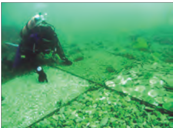
Fig.2: Photograph of diver inspecting 1m 2 experimental settlement plots (clockwise from top: 20mm stone, scallop shell, 50mm stone, crushed whelk) one month after deployment within the Poole Bay artificial reef site.
