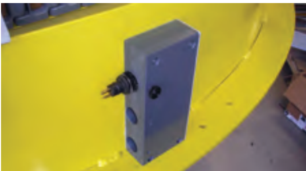
Figure 4: Housing containing 3 optical turbidity sensors; note each sensor looks across the flume channel.
