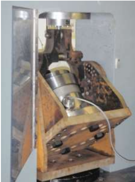
Figure 3.4 Calibration of tri-axial loadcell
