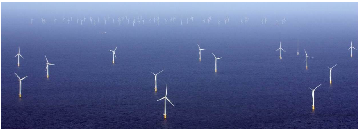
Figure 3. A bird's eye view of OWEZ in the foreground and PAWP in the background. Note difference in turbine density and the meteo mast on the far right of OWEZ. Photo Hans Verdaat, IMARES, 7 July 2010.
