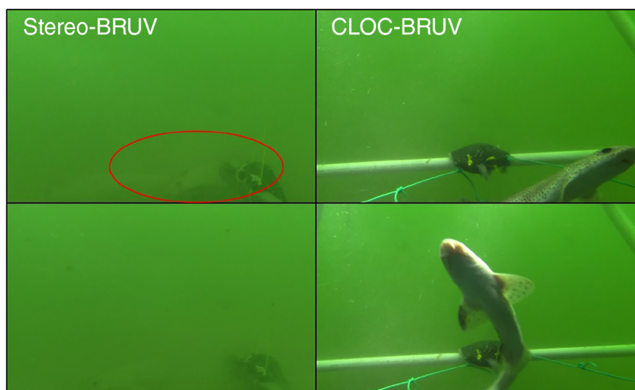
Fig. 6. Observations of a taxa taken from comparative simultaneous deployments without the CLOC (left) and with the CLOC (right) where a lesser spotted dogfish is visible in a location of low underwater visibility (3.5 m) in Swansea Bay, South Wales. An individual is also present in the imagery without the CLOC; however, distinguishing features are difficult to determine.
