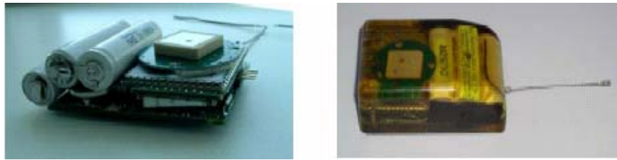
Figure 6.32. GPS/GSM-transmitter (prototype) before and after encapsulation in epoxy resin. Length of transmitter (excl. antenna) 60 mm.
