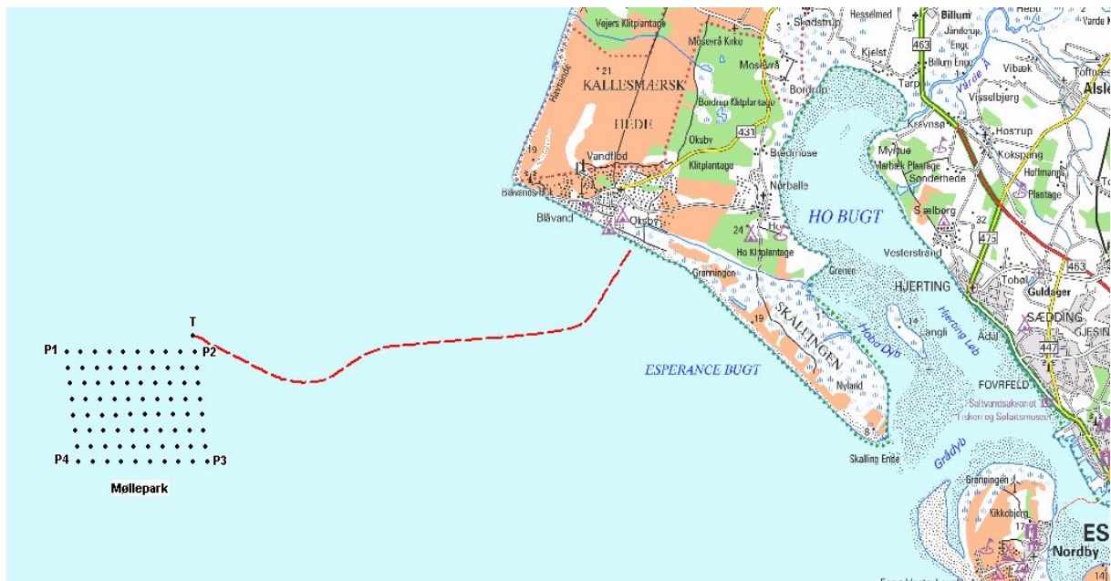
Figure 5.1. The offshore wind farm at Horns Rev and the cable trace to land at Hvidbjerg Strand. T marks the transformer platform.
