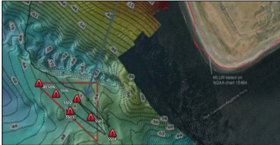
Figure 5. Target locations of autonomous acoustic instrument package deployment locations and three additional ADCP instrument deployments. The SnoPUD tidal turbine site is outlined with the red triangle and the proposed cable run is outlined in blue, all overlaid on a bathymetric map of the area.
