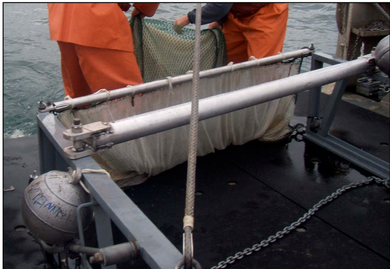
Figure 3: Beam trawl used for collecting epifaunal invertebrates and groundfish.
