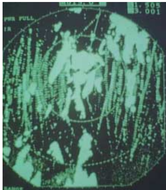
Figure 14. Scanning radar screen during intense migratory activity, spring 1996.
