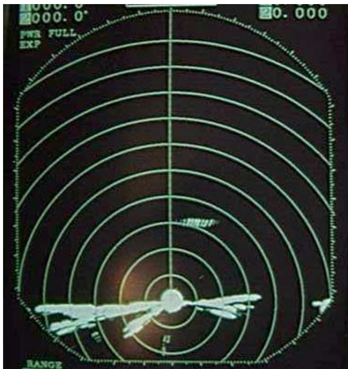
Figure 10. Display screen of vertical radar during autumn 1995 monitoring. Light horizontal area at bottom is ground level. Top is straight up, right is west. Distance between concentric rings is 0.25 nm (463 m). Signature in center, touching third range ring is signature of a bird(s) 1322 m (4340 ft) in altitude above radar. Detection range above radar was 5.1 km (16,732 ft) AGL.
