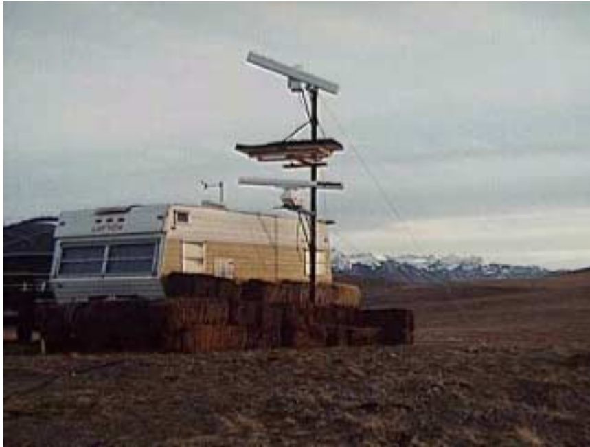
Figure 6. Scanning and vertical radar pedestal mount for interference management.
