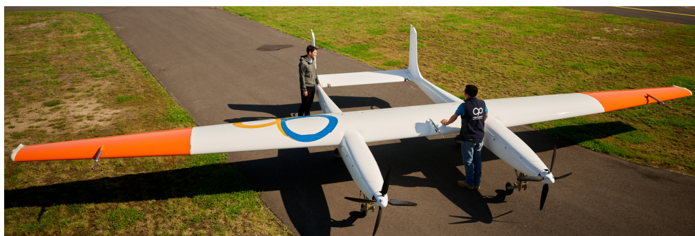
Figure 2. Ampyx Power’s AP3 with a wingspan of 12 m and a wing surface area of 12 m 2 during runway testing at Breda International Airport in May 2021 (photo courtesy of Ampyx Power B.V.).
