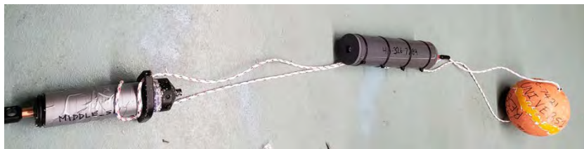
Figure 5. Photograph of the mooring with the acoustic release at the bottom (on the left of the image), the LS1 acoustic recorder in the center of the line, and a sub-surface buoy at the top (on the right).
