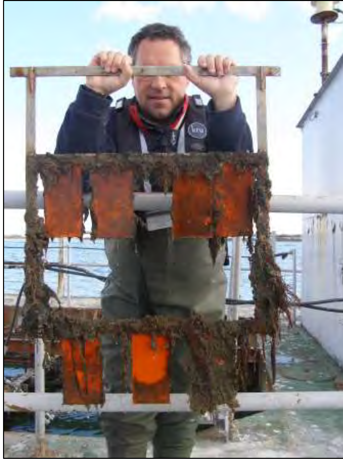
Figure 15: Example of a settlement frame with plates.
