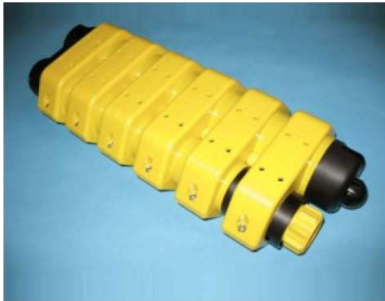
Figure 6: The Geospace OBX Ocean Bottom Recorder containing a 3-axis geophone and a low sensitivity hydrophone. Five of these systems are proposed to be deployed.
