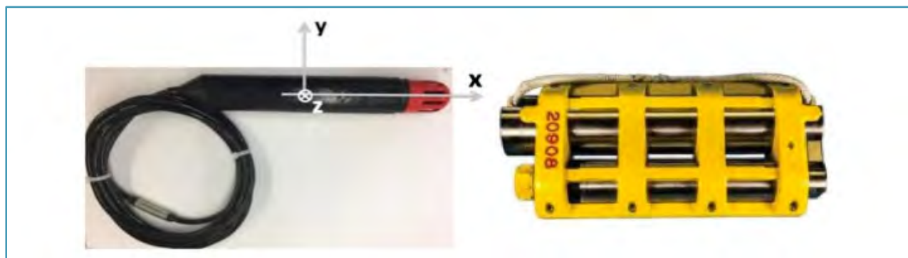
Figure 6. Close up view of the three-axis geophone (right panel) and OBX system (left panel)
