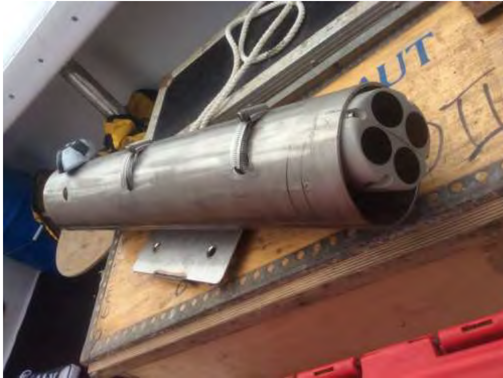
Figure 9: Fugro scour monitor acoustic device.
