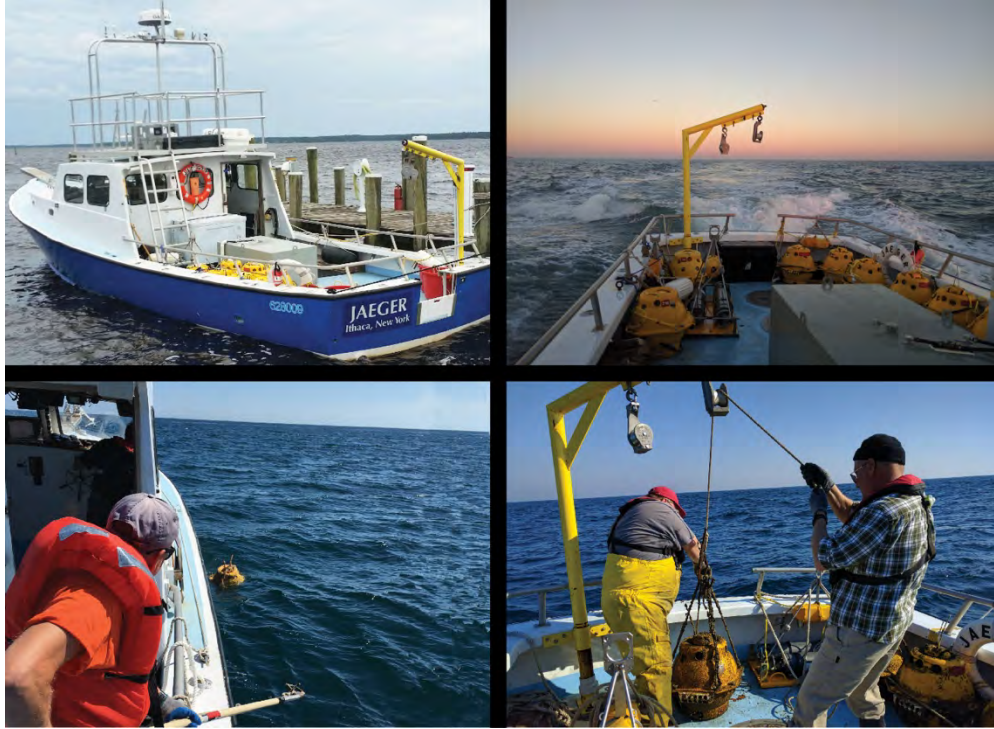
Figure 2. Field operations photographs shown as: A) Cornell’s research vessel used for deployment and recovery of recording equipment, the R/V Jaeger. B) The deck of the R/V Jaeger loaded with MARUs and AMARs. C) A field technician recovers a MARU. D) The recovered MARU is hauled on deck. Photo credits: Fred Channell (A); Kristin Hodge (B, C, D).
