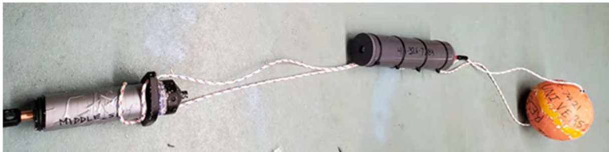
Figure 8. Photograph of the mooring with the acoustic release at the bottom (left side of image), the LS1 acoustic recorder in the center of the line, and a sub-surface buoy at the top (right side of image).
