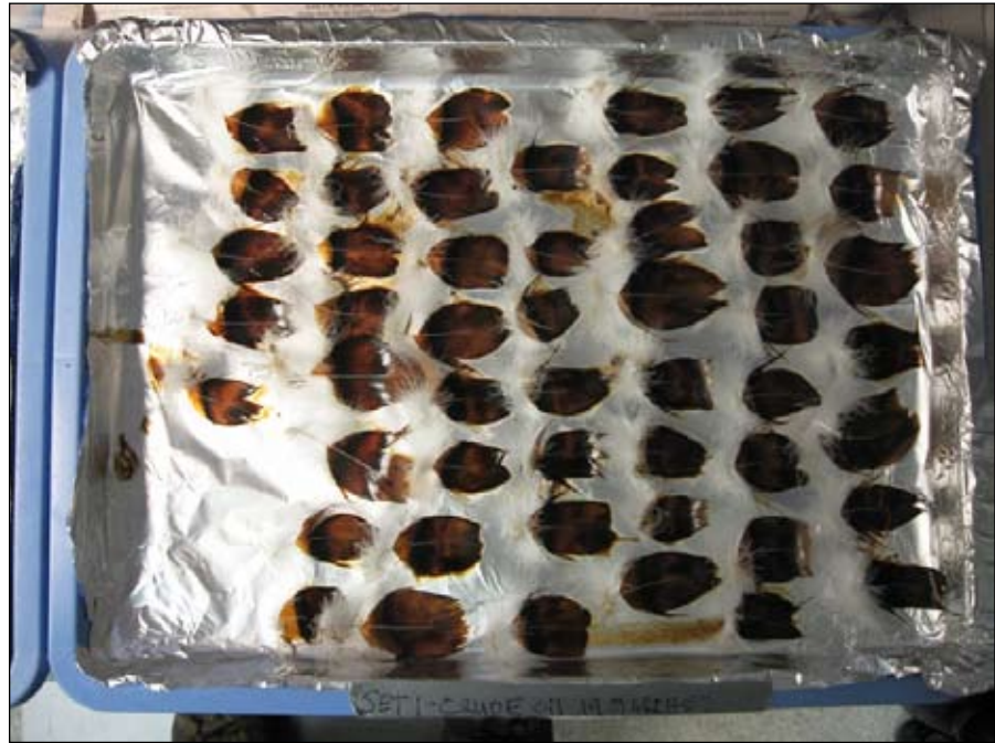
Figure 1. An example of contaminated feathers on an aluminum-foil covered tray. Feathers would remain like this for one hour to three weeks depending on which time trial was being tested for the contaminant.
