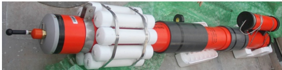
FIGURE 8. UH-DEVELOPED AMP-1 HYDROPHONE STATION.
