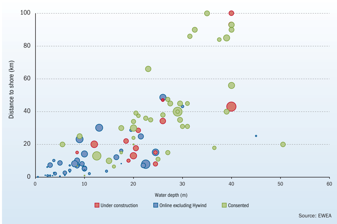
FIGURE 1.17 DISTANCE AND DEPTH OF ONLINE, CONSENTED AND UNDER CONSTRUCTION OFFSHORE WIND FARMS
