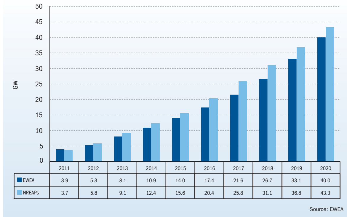
FIGURE 1.7 PROJECTED CUMULATIVE OFFSHORE WIND CAPACITY (EWEA AND NATIONAL RENEWABLE ENERGY ACTION PLANS)
