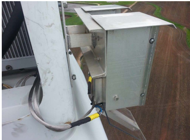
Figure 3-1 ReBAT® acoustic detectors deployed on a wind turbine nacelle at BSGF showing the reflector plate on the upward looking detector
