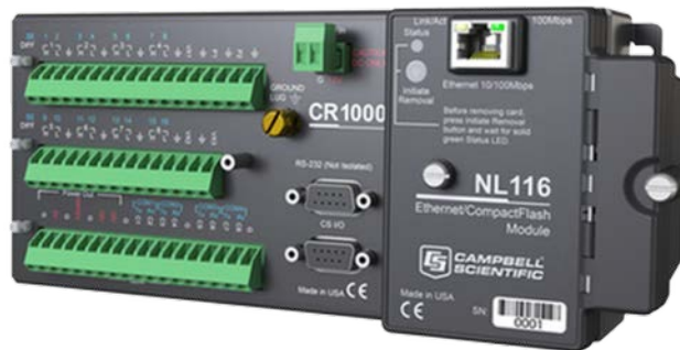
Figure 5-2 Campbell Scientific CR1000 datalogger with NL-116 (NL-120 was used) Ethernet option (cover removed)
