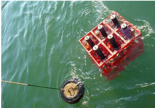
Fig. 2-18: Plastic frame for inter calibration experiments with 6 T-PODs during recovery.
