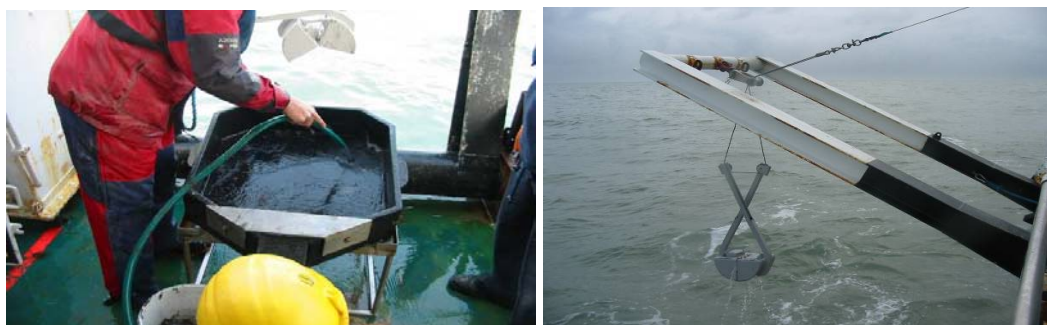
Figure 2. Van Veen sampling on board of Belgica RV and sieving over a mm sieve (before fixation of the sample) (photo's Marijn Rabaut).
