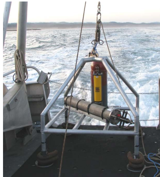
Figure 2-5. Hydrophone Mounted on Lander Prior to Deployment
