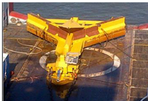
Figure 5.3 - SCAR plough configured for boulder clearance operations.
