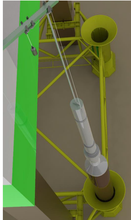
Figure 5.8 – Example of a piling hammer (with follower) and subsea hammer on pile and piling through the PIF
