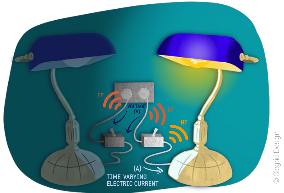
Fig. 1 Illustration of the example of the lamp and the units of measurement used to define electric current – Voltage (in V) and intensity (in A). Adapted from RTE 1 .
