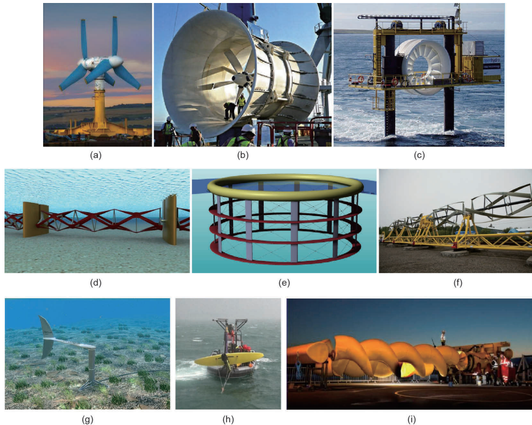
Fig. 4. Examples of tidal and ocean current devices. (a) Atlantis AK1000 axial-flow turbine (1 MW) [31]; (b) Atlantis Solon-K ducted turbine (1 MW) [32]; (c) OpenHydro open-center turbine (250 kW) [33]; (d) Kepler transverse horizontal axis water turbine (THAWT), a kind of cross-flow turbine (4 MW) [34]; (e) Edinburgh vertical axis cross-flow turbine concept (100 MW) [35]; (f) Gorlov helical turbines before deployment at Cobscook Bay, ME, USA [36]; (g) bioSTREAM (150 kW) oscillatory-hydrofoil turbine (image courtesy of BioPower) [37]; (h) Minesto deep sea tidal kite [38]; (i) Flumill Archimedes screw turbine [39].
