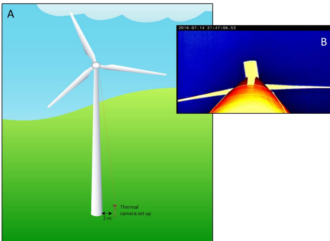
Figure 5: A depicts thermal camera set-up from 2 m from the wind turbine base at Wolf Ridge Wind, LLC. B shows the field of view from the thermal camera. Note the screen was centered where the tower meets the nacelle in order to establish a field of view that includes 10 m from the ground up to the nacelle.
