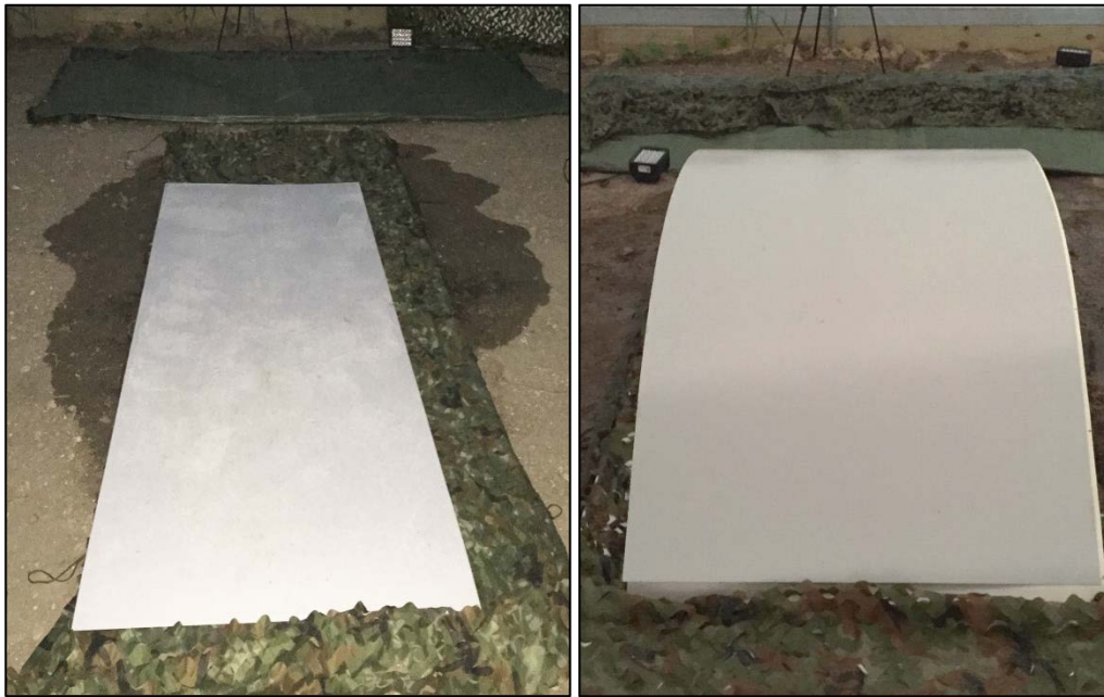
Fig. 10: Placement of treatment surfaces over the water tray. The left image shows the treatment surface aligned with the right edge of the aluminum plate and camouflage netting over the water tray. The right image shows the treatment surface being placed on top of the turbine tower section.
