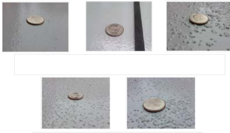
Figure 1: Range of experimental surface textures (including one applique) that were used in the flight facility testing in 2015.
